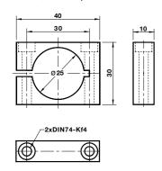
(incl.2 fastening screws M4x35 DIN912 VA)
